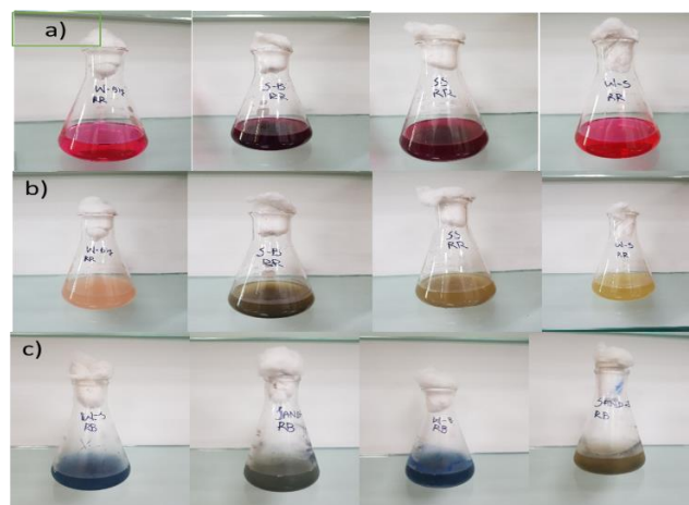
Figure 1. a) Reactive Red dye supplemented media before inoculation b) Reactive Red dye supplemented media after 72hrs inoculation c) Reactive Blue dye supplemented media after 72hr inoculation.
