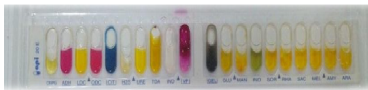
Fig 1: API strip showing different result after incubation confirming presence of E. coli .
