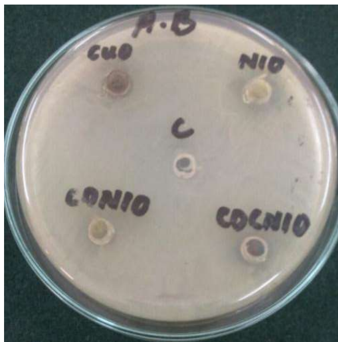
Fig. 4(d): Zone of inhibition of nickel oxide, copper oxide and copper doped nickel oxide NPs against Pseudomonas aeruginosa
