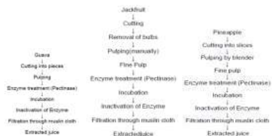
Fig 6: Extraction of juices using pectinases in the enzymatic liquefaction process (Compiled from Ahmed et al., 2014).
